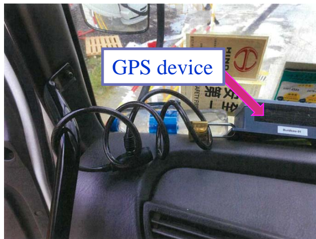
All dump trucks equipped with GPS system
